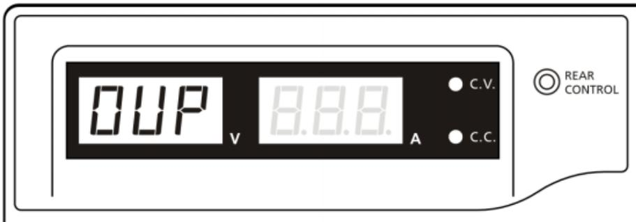
Figure 13 - Overvoltage Protection
