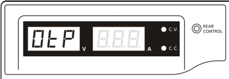
**Figure 14 - Overtemperature Protection**
