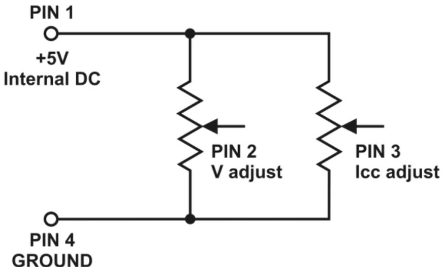
Figure 6 - Variable 5 k $\Omega$  Resistors Setup
