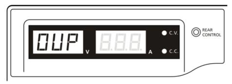
Figure 13 - Overvoltage Protection
