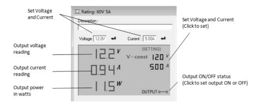
Figure 7 - PC Software General Functions and Display
