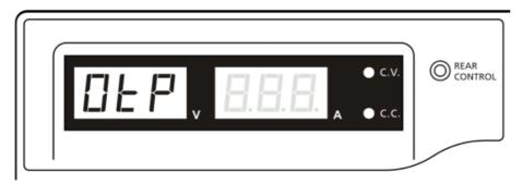
Figure 14 - Overtemperature Protection
