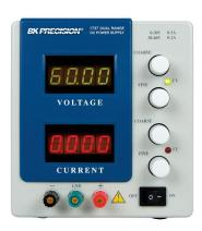
B&K Precision's models 1737 and 1747 are general purpose dual range DC power sources. These power supplies can output higher voltage at a lower current range or more current at a lower voltage range. Two 4-digit LED displays continuously monitor the output voltage and current. The power supplies can be operated locally from the front panel or remotely through the RS-232 interface.
