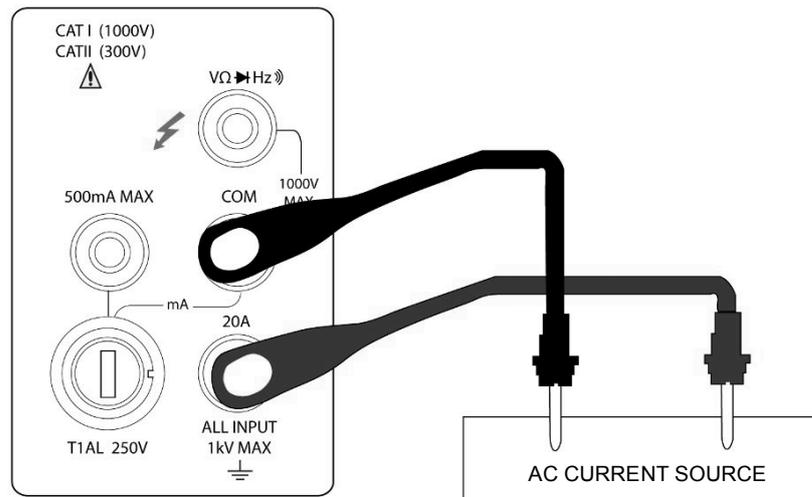
**(Model 2831E) AC Current measurement on Range: 2 A, 20 A**
