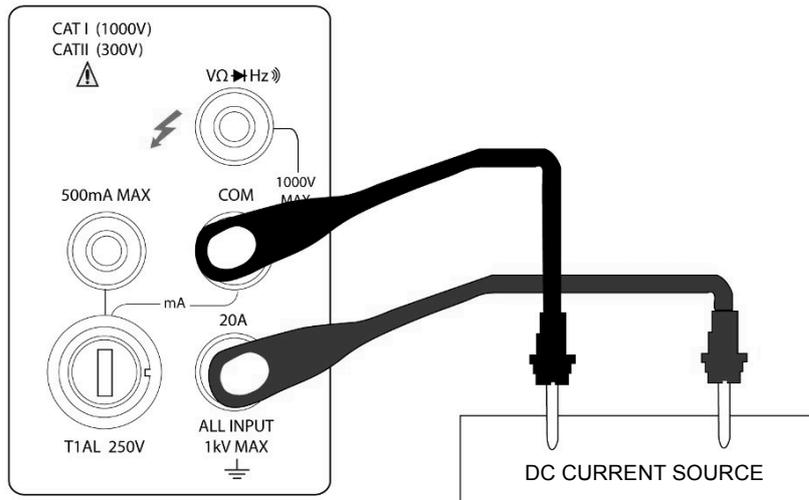
**(Model 2831E) DC Current measurement on Range: 2 A, 20 A**
