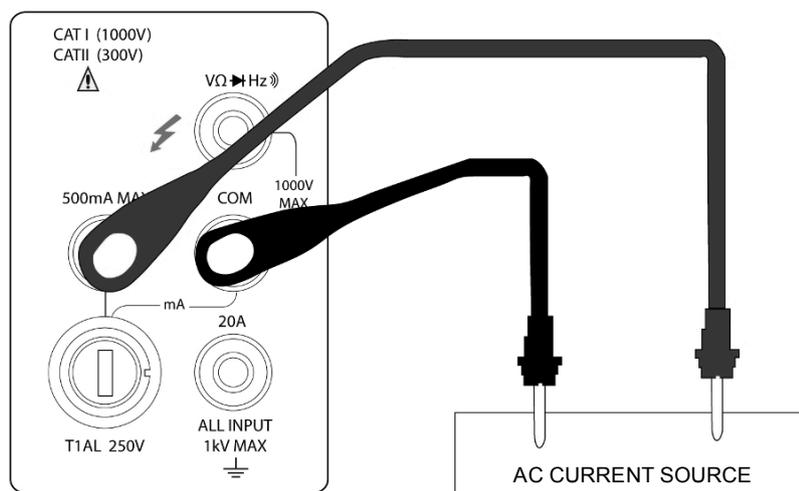
**(Model 2831E) AC Current measurement on Range: 2 mA, 20 mA, 200 mA**
