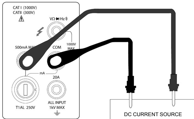
**(Model 2831E) DC Current measurement on Range: 2 mA, 20 mA, 200 mA**
