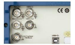
Use the external 10 MHz clock input and output to synchronize your signals to a master time base. The Sync output generates a TTL pulse for synchronization to a channel's frequency. An external trigger BNC connector is also available for inputting or generating a trigger signal.
