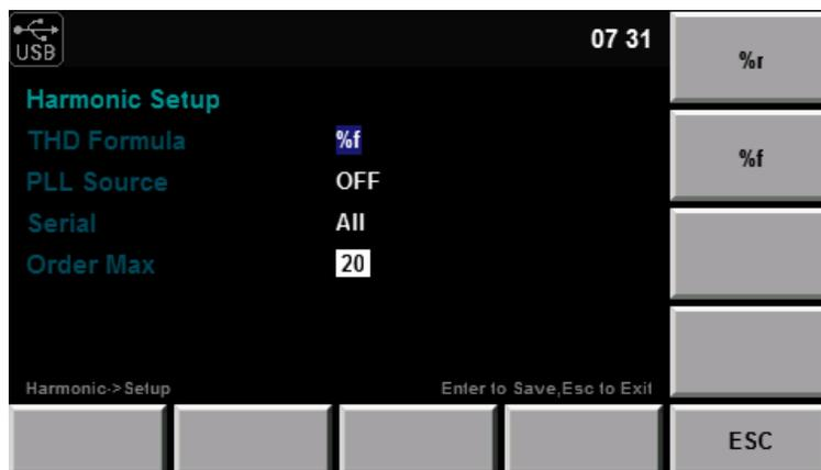
Figure 6.1: Harmonic Measurement Setup Menu
