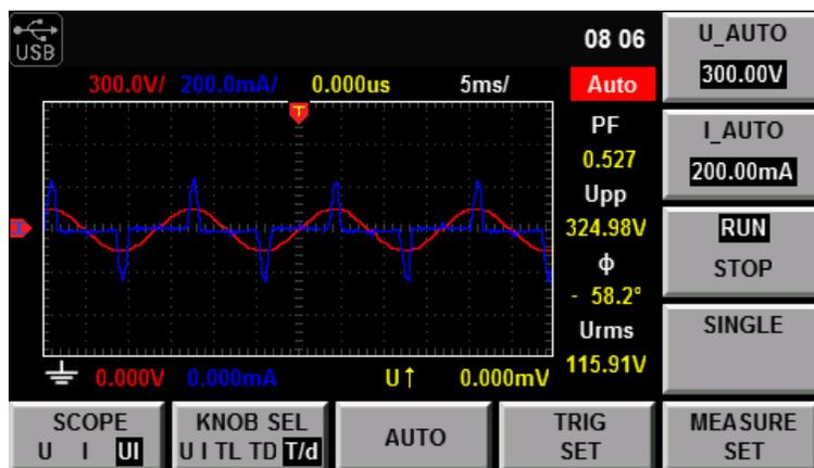
Figure 5.1: Waveform Display Details
