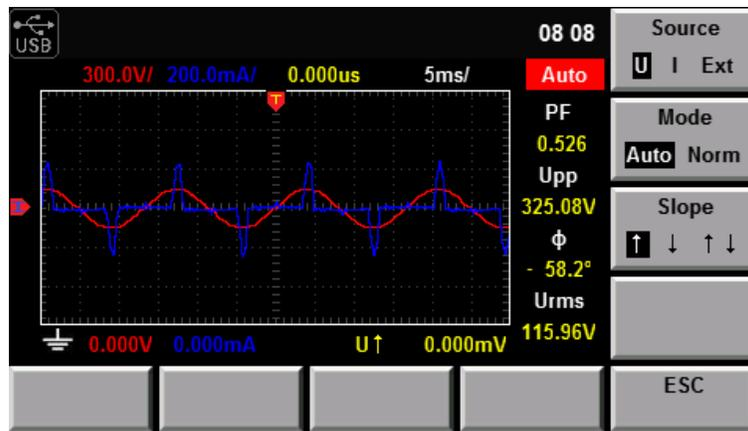
Figure 5.2: Trigger Setup Screen
