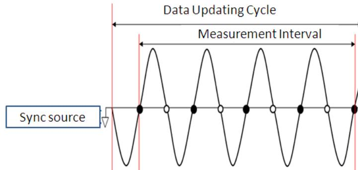
Figure 3.1: Measurement Timing
