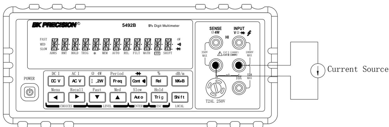
**For low current measurement: INPUT LO and SENSE LO terminals are used.**
