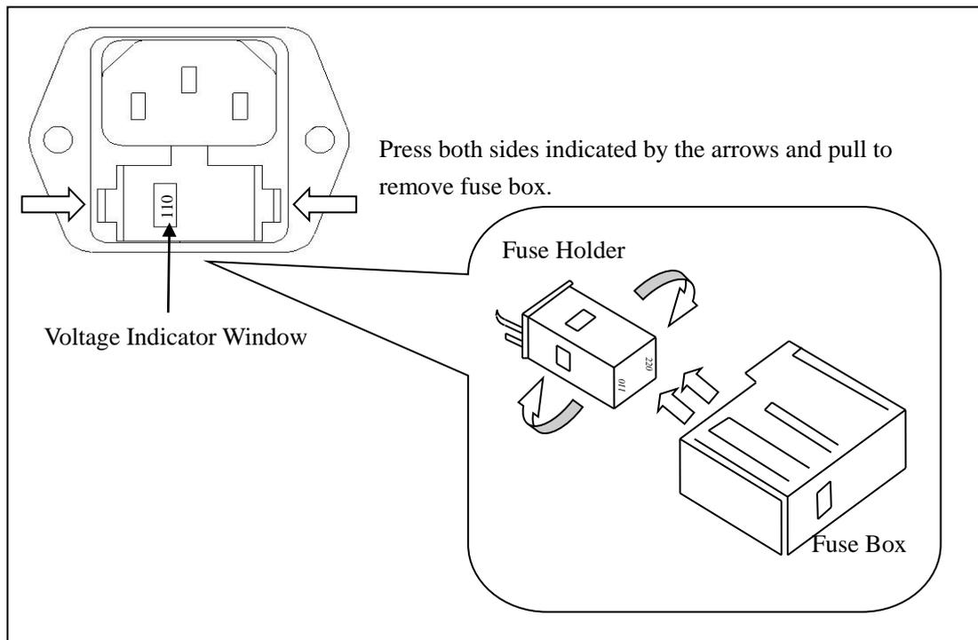
There is a second fuse with a fuse holder located in the front panel of the multimeter. This is an over current protection fuse for the low current measurement input. It is rated for a T2AL, 250 V fuse. To remove and replace this fuse, see the illustration below:
