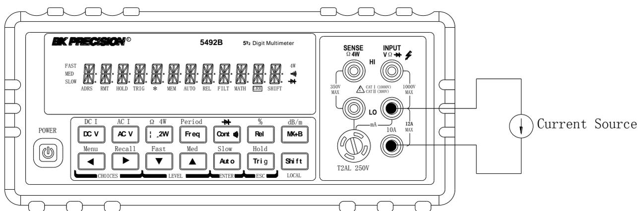
**For 1 A or higher current measurement: 10 A and INPUT LO terminals are used.**
