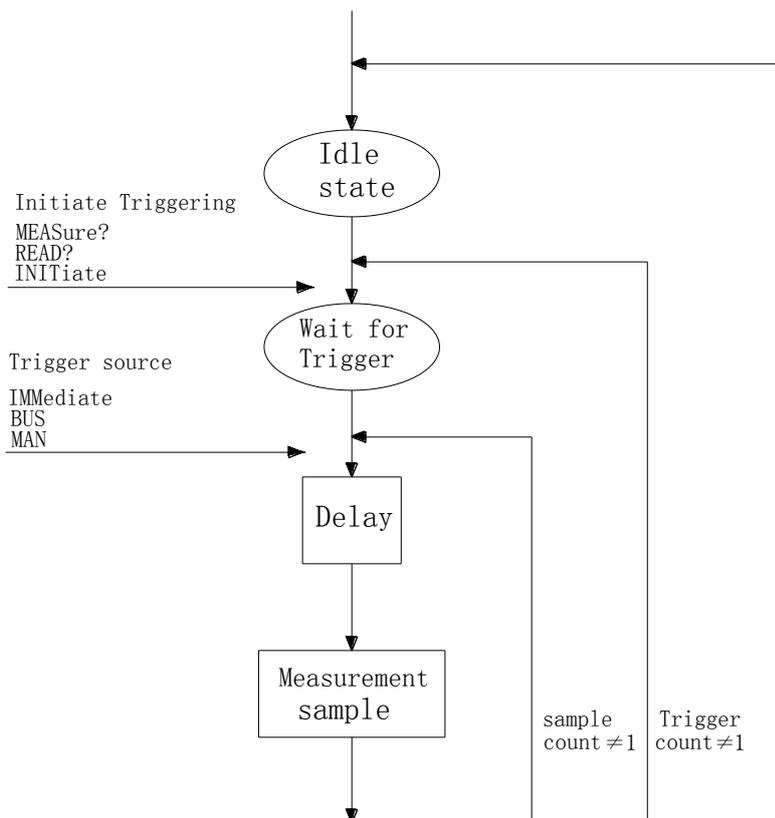
Figure 4-2 Trigger model
