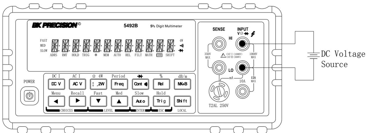
Input Resistance = 10 MΩ on 1000 V and 120 V ranges;
