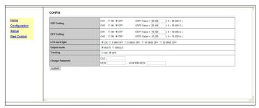
Control settings page for configuration of protection and password settings for the system
