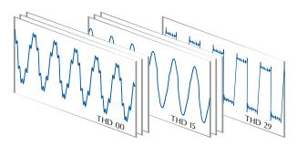
Select from 30 built-in THD (total harmonic distortion) waveforms
