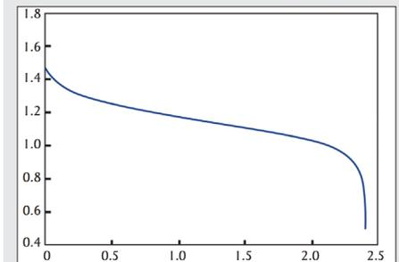
The built-in battery test function uses CC mode to calculate the battery capacity using a fixed current load discharge. Users can specify cut-off voltage level, capacity level and time stop conditions.
