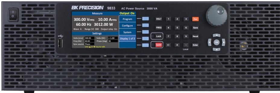
The 9830 Series are low distortion, single-phase AC power sources delivering a maximum of 3000 VA, 300 Vrms, 30 Arms / 97.5 Apk with the output frequency adjustable from 45 Hz to 1200 Hz. Housed in a compact 3U form factor, the AC source is capable of generating both AC, DC, and AC+DC output.
