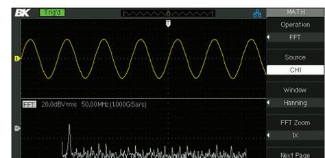
Display and measure the input signal's frequency spectrum. Select one of the 4 FFT windows: Rectangular, Hanning, Hamming and Blackman. Use cursors to measure the spectral component's magnitude and frequency.
