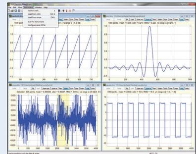
Use WaveXpress to easily generate, edit, and upload custom arbitrary waveforms to the generator via the remote interface. Generate waveforms in the software by importing a text file or define via freehand, point draw, and waveform math functions.
