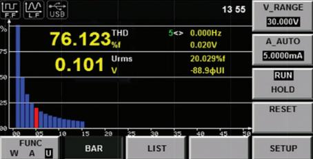
The parameters of each harmonic measured can be displayed in a bar chart.
