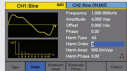
Generate up to 10 harmonics with independent amplitude and phase settings.
