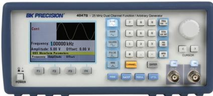
The 4047B is a versatile dual channel 20 MHz function generator with arbitrary waveform capability. It features a true point-by-point AWG (arbitrary waveform generator) architecture to produce accurate and precise arbitrary waveforms combined with a DDS architecture offering easy-to-use conventional function generator capabilities.
