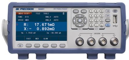
The BA6000 Series Battery Analyzers use a 1 kHz AC constant current source to measure the battery's impedance expressed by 11 different measurement functions. With a basic voltage and impedance accuracy of 0.1% and micro-ohm resolution, these instruments are well-suited for analyzing a wide range of battery types and configurations in the lab, quality control and manufacturing environments.
