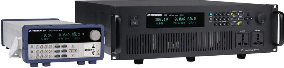
The 9800 Series is both a programmable AC source and measurement tool. These fully programmable linear AC sources deliver a maximum of 1500 VA through the universal line output terminals on the front and the output connector on the rear.
