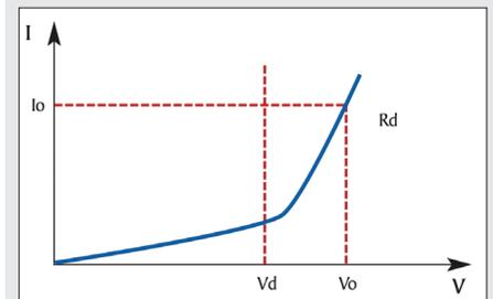
Use the load's unique CR-LED operating mode to test LED drivers. This function allows users to configure the LED's operating resistance and forward voltage to simulate the loading behavior of typical LEDs.
